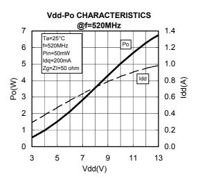
RoHS Compliance, Silicon MOSFET Power Transistor 175MHz,520MHz,2W
